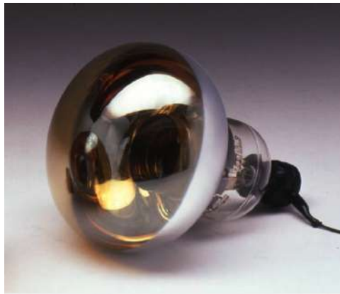
Figure 1.7: Photo of a single photo-sensor for Hyper-Kamiokande.
